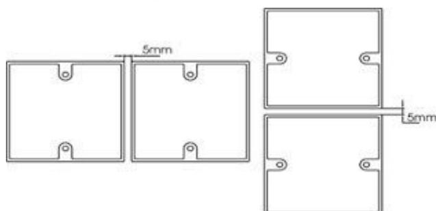
*Figure depicting the distance buried negative substrate for square switches*
