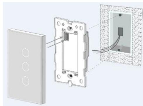
**Step 3:** Secure the bottom part onto a junction box with screws, and then mount the touch panel back.
