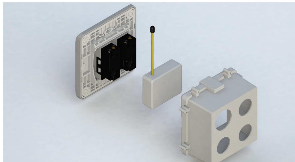
1. put the in wall switch into a wall box and connect the AC power wire L,N to PAN04 connector L, N.
