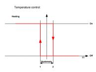
When the temperature is decreasing and reaches point 1 (defined by parameter 43), heating is turned on and remains active until the temperature in the room is not increased to reach point 2 (defined by parameter 44). In this moment heating is turned off.
