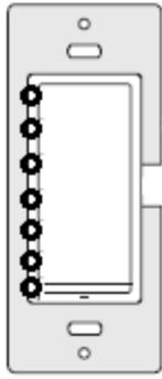
All 7 LED indicators are ON when the connected lighting is at full brightness (100%)
