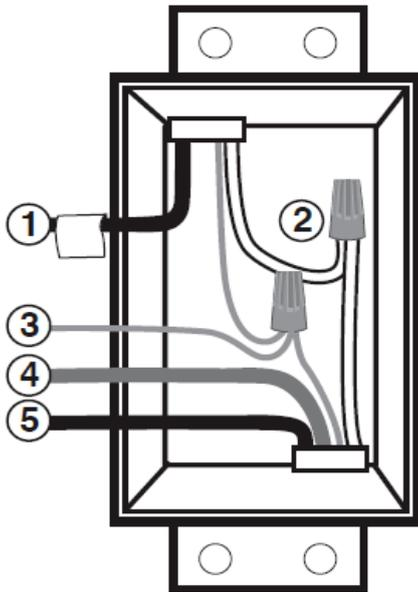
4 wires for 2-way circuit
