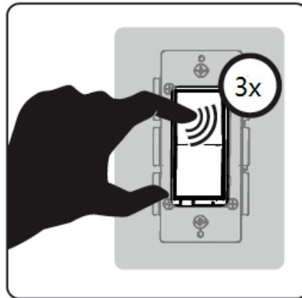
2. Quickly tap the top side(ON) of the rocker 3 times
