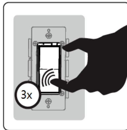
Then, quickly tap the bottom side(OFF) of the rocker 3 times
