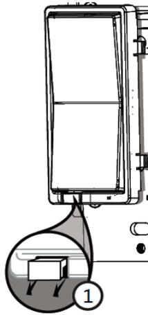
1. Lift the activator up to avoid electrical shock
