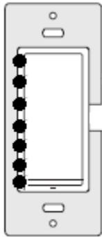
All 7 LED indicators are OFF when the connected lighting is shut off (0%)
