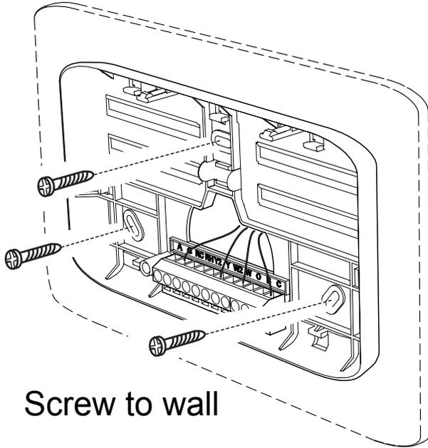
1. Hold the CT110 wall plate against the wall, with the wires coming through the hole in the wall plate.
