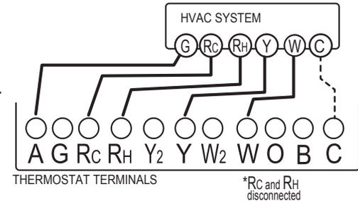
**3 Wires** **C Wn Yn RH G** **Multi-stage Heat and Multi-stage Cool**
