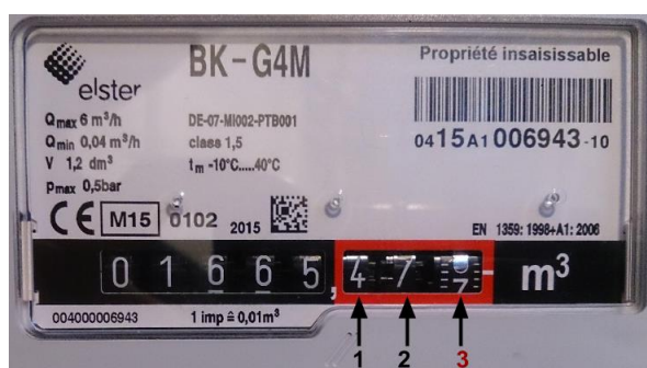
Figure 1: Determining the index of red digit with silver spot
