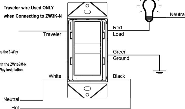
For 3-Way installation, the ZW15SM-N requires the 3-Way Control Auxiliary Switch ZW3K-N.
