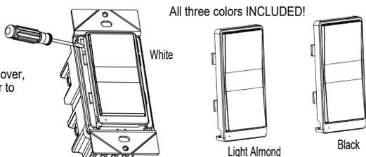
To Replace the Face Cover, use a small screwdriver to pry off the cover
