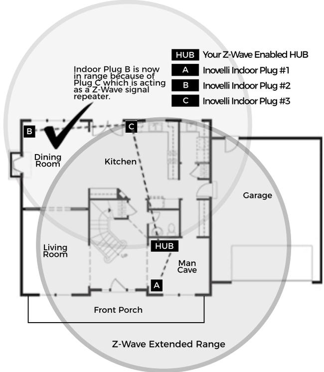
In this example, "Plug B" is out of range and will not work unless either the HUB is moved or a Z-Wave repeater is installed.
