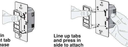
After frame is removed, remove existing push buttons by pressing out buttons from back of frame and replace them with desired color change push buttons by pressing in from front of frame. To make IR capable, use new DIM/BRIGHT button with IR window.
