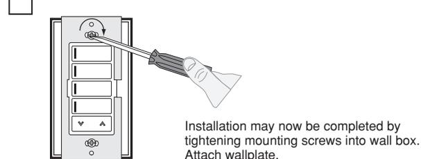
Installation may now be completed by tightening mounting screws into wall box. Attach wallplate.
